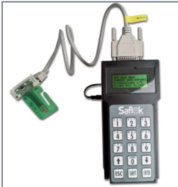
Handheld (LPI) with Smartcard probe connected
