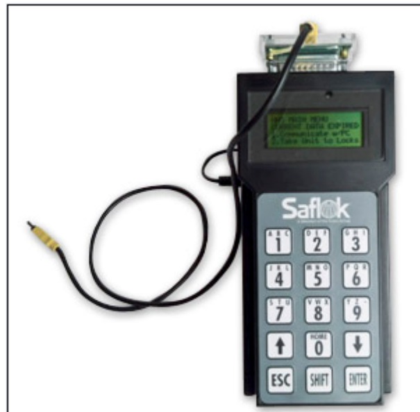
Handheld (LPI) with RFID probe connected
