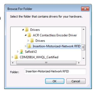
Windows will then prompt you to install the driver for the USB Serial port. Windows will need the drivers for it as well. Browse to the Insertion-Motorized Network RFID.. folder on the CD again.
