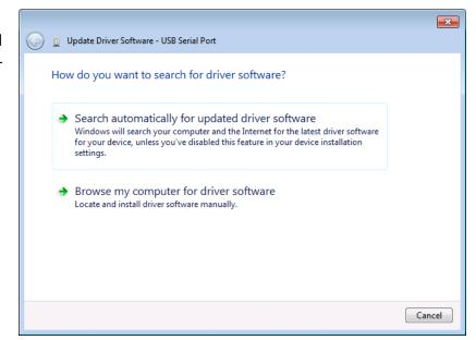
After the driver installation is completed, check the device manager to determine which COM port it is on. Click the Windows Start button, then Control Panel. Select to View By: Large Icons. Double click Device Manager.
