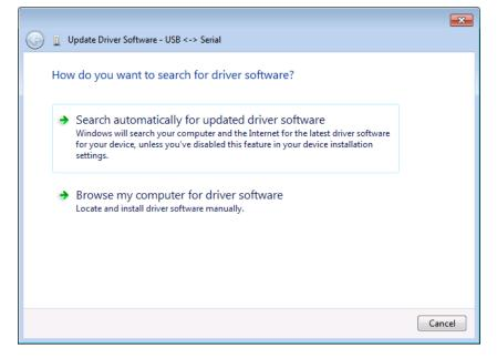
If needed, the USB drivers are located on the Saflok Program installation CD, in the Drivers folder. Select the appropriate driver folder based on the host computer's operating system and the USB <-> Serial converter will then be installed. Windows 7 or later will usually install the drivers automatically.
