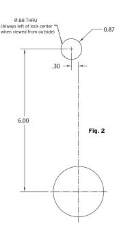
Note: The hole shown above is not located on the drill fixture. Use these measurements to locate the hole.
