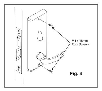
13. Secure the inside trim cover to the inside trim using two M4 x 16mm Torx screws (see Fig. 4).
